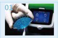
**Specimen Adding** Input the user information, and add the sample to be tested.
